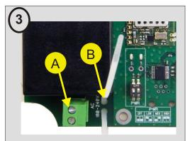
Connect the 230V (A) and secure the powercable with the tie-wrap (B). Apply the power.
