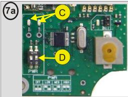
You can adapt the transmission power with two DIP switches (D). LEDs (C) allow you to check your setting.
