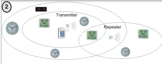
The DHF repeater V2 (ref.: 927241) enables to extend an area non covered by the main DHF transmitter.
